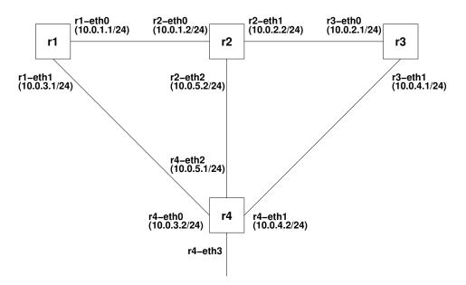
Use the addHost() and addLink() API functions. Establish connectivity between neighbors using the IPv4 addresses shown above and using static routes.
