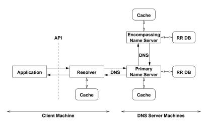
The resolver is typically tightly integrated into the operating system (or more precisely standard libraries).
