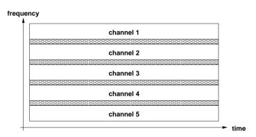
• Signals are carried simultaneously on the same medium by allocating to each signal a different frequency band
