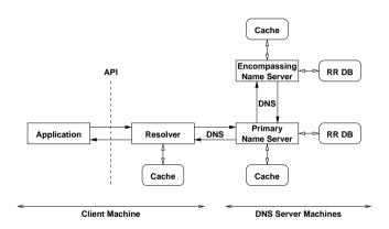
• The resolver is typically tightly integrated into the operating system (or more precisely standard libraries).
