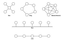
• The *topology* of a network describes the way in which nodes attached to the network are interconnected
