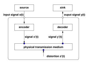
• Signals are in general modified during transmission, leading to transmission errors.
