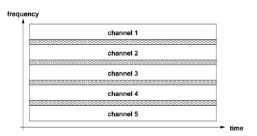
Signals are carried simultaneously on the same medium by allocating to each signal a different frequency band
