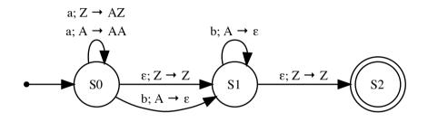
Pushdown automata can be represented as graphs where nodes (circles) represent states, arrows represent state transitions, an arrow pointing from a small black circle indicates the initial state, and accepting states are marked with with a double circle.
