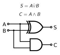
The gate delay  $t_g$  is the time it takes for the output signal to be a stable reflection of the two input signals. Assuming that every gate has the same gate delay, the half adder works with a constant gate delay of  $t_{ha}=t_g$ .
