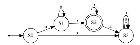
• State machines can be represented as graphs where nodes (circles) represent states, arrows represent state transitions, an arrow pointing from a small black circle indicates the initial state, and accepting states are marked with with a double circle.
