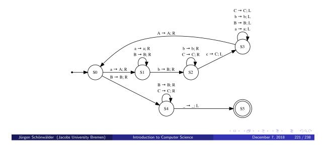
There is no common graphical notation for Turing machines. We label transitions using the symbol under the head, an arrow pointing to the symbol written under the head, and a semicolon followed by the movement indicator (L = left, R = right).
