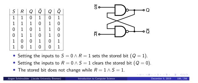
The  $\bar{S}\bar{R}$  latch behaves like an SR latch except that the input signals are inverted: The latch does not change as long as both S and R are high. If S goes low while R remains high, the bit in the latch gets set to high. Similarly, if R goes low while S remains high, the bit in the latch gets cleared. S and R should not go together low.
