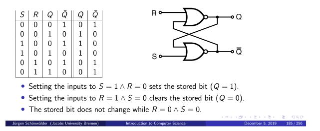
The SR latch has two inputs S and R and two outputs Q and  $\overline{Q}$ . The outputs Q and  $\overline{Q}$  feedback into the circuit and hence the value of the outputs Q and  $\overline{Q}$  depends on the two inputs and the previous values of Q and  $\overline{Q}$ . We can write this as
