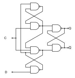
A common symbol for a positive edge triggered D flip-flop is show below:
