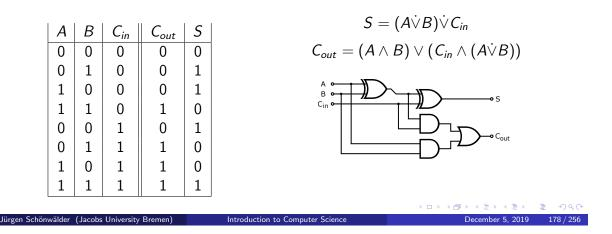
Assuming that every gate has the same gate delay  $t_g$ , the full adder works with a constant gate delay of  $t_{fa} = 3 \cdot t_g$ . Note that the carry in signal only has a gate delay of  $2 \cdot t_g$  to the carry out signal. Further information:
