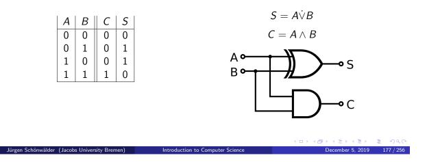
The gate delay  $t_g$  is the time it takes for the output signal to be a stable reflection of the two input signals. Assuming that every gate has the same gate delay, the half adder works with a constant gate delay of  $t_{ha} = t_g$ .
