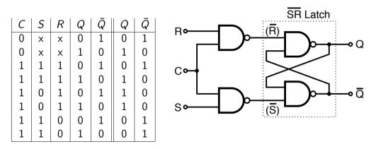
• The control input *C* enables the SR latch.
