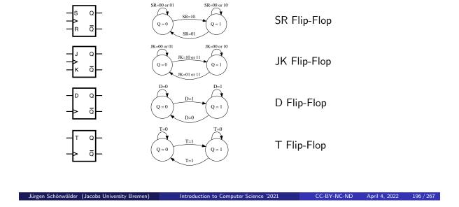
All flip-flops are edge triggered on the clock input C.
