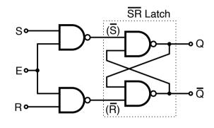
• The control input E enables the latch, the latch does not change while E is low.
