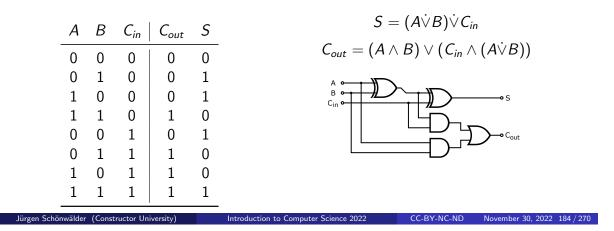
Assuming that every gate has the same gate delay  $t_g$ , the full adder works with a constant gate delay of  $t_{fa} = 3 \cdot t_g$ . Note that the carry in signal only has a gate delay of  $2 \cdot t_g$  to the carry out signal.
