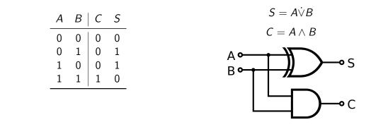
The gate delay  $t_g$  is the time it takes for the output signal to be a stable reflection of the two input signals. Assuming that every gate has the same gate delay, the half adder works with a constant gate delay of  $t_{ha} = t_g$ .
