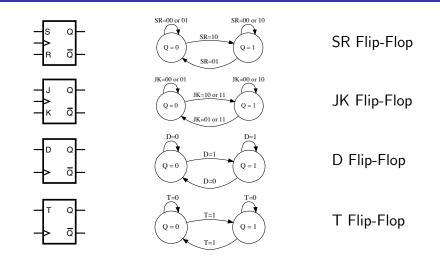
All flip-flops are edge triggered on the clock input C.
