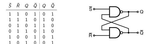
• Setting the inputs to  $\bar{S} = 0 \land \bar{R} = 1$  sets the stored bit (Q = 1).
