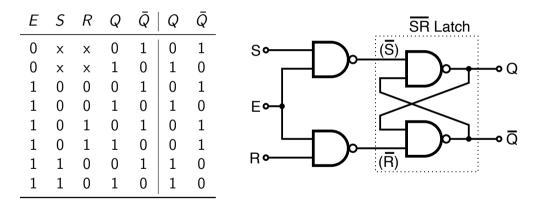
• The control input E enables the latch, the latch does not change while E is low.
