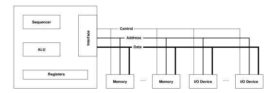
Today's common computer architecture uses busses to connect memory and I/O systems to the central processing unit
