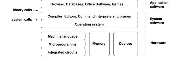
From the operating system perspective, the hardware is mainly characterized by the machine language (also called the instruction set) of the main processors, the memory system, and the I/O busses and interfaces to devices.
