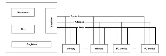
Today's common computer architecture uses busses to connect memory and I/O systems to the central processing unit
