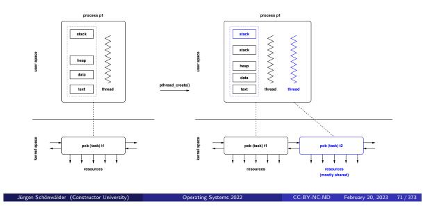
This slide aims to explain the effect of the pthread\_create() call. The following happens if a process with its own memory image and thread of control invokes the pthread\_create() call (which usually is a wrapper around a system specific system call):
