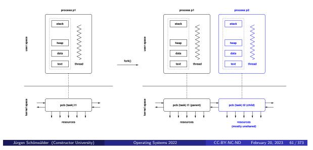
This slides aims to explain the effect of the fork() system call. The following happens if a process with its own memory image and thread of control invokes the fork() system call:
