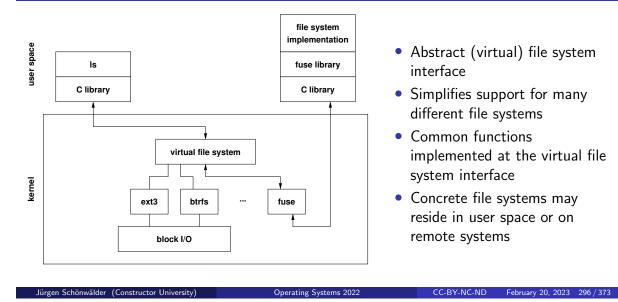
On Linux, the virtual file system is defined by structures containing function pointers for the different file system operations (see <linux/fs.h>)
