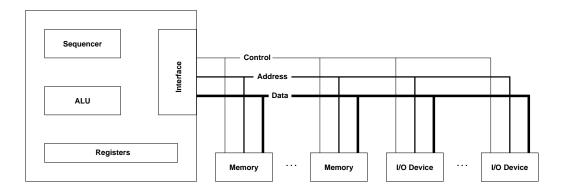
Today's common computer architecture uses busses to connect memory and I/O systems to the central processing unit (CPU)
