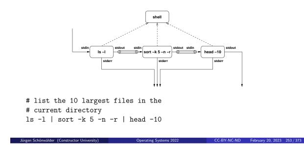
Pipes are kernel objects that support unidirectional communication from the write end of a pipe to the read end of a pipe. When the kernel creates a new pipe, it allocates two new file descriptors for the two endpoints of the pipe in the file descriptor table.
