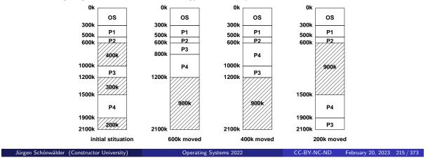
If a memory allocation system is suffering from too many small external fragments, one could come up with the idea to compact memory again by moving memory segments around in memory. Relocating memory is of course expensive and the costs depend on how memory is moved. Finding a good compaction strategy that minimizes the memory moved can be tricky.
