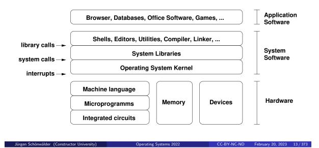
From the operating system perspective, the hardware is mainly characterized by the machine language (also called the instruction set) of the main processors, the memory system, and the I/O busses and interfaces to devices.
