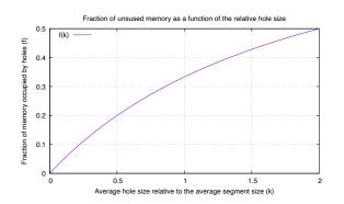
$\implies$  As long as the average hole size is a significant fraction of the average segment size, a substantial amount of memory will be wasted
