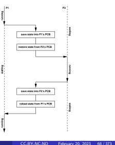
A context switch is the process of storing the state of a process or thread, so that it can be restored and resume execution at a later point. Context switches happen frequently and hence it is important that they can be carried out with low overhead.
