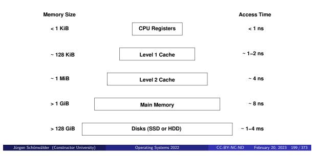
In the following, we will focus on the main memory. Organizing the usage of the available physical memory is a key function of an operating system. A mismatch of the memory management strategies used by an operating system kernel with the assumptions made by the developer of an application can slow down applications significantly.
