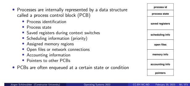
In the Linux kernel, the process control block is defined by the C struct task\_struct, which is defined in include/linux/sched.h. It is a very long struct and it may be interesting to read through its definition to get an idea how central this structure is for keeping the information related to processes organized in the kernel.
