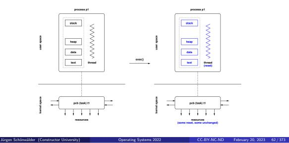
This slides aims to explain the effect of the exec() system calls. The exec() system calls load a new process image. This essentially means that the running program is replaced by another program. Hence, all memory segments of the process invoking the exec() system call are loaded (text and data) from an executable file or reset (heap and stack). Furthermore, the thread of control is reset to start from the entry point of the newly loaded program.
