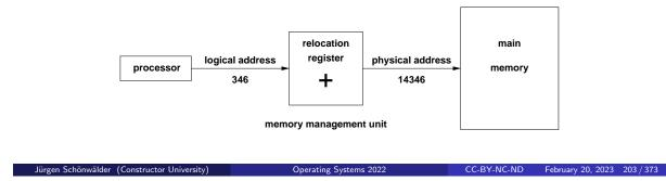
The simplest form of a memory management unit is to use a relocation register that provides a value that is added to logical addresses in order to obtain the corresponding physical addresses.
