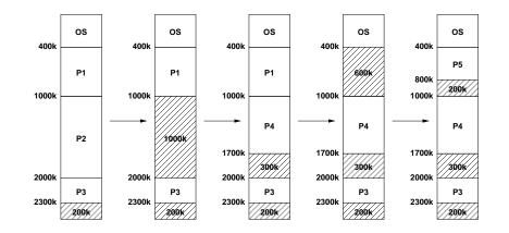
• In the general case, there is more than one suitable hole to hold a new segment — which one to choose?
