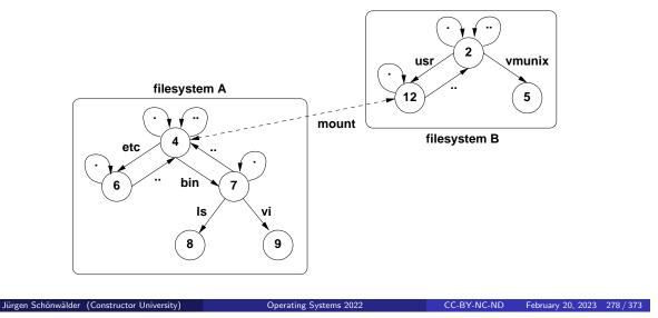
Mounting is the process of making a directory from another file system (usually residing on some other storage system) available as part of a local file system name space. Mounting allows to build logical file system name spaces that span multiple devices. Note that the mounted file systems may be of different file system types. Mounted file systems may also reside on remote systems.
