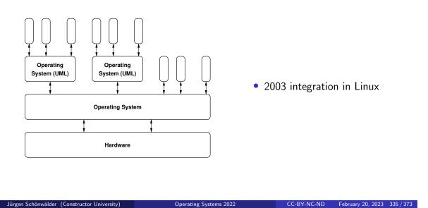
User-mode linux is not a very efficient virtualization solution and it had for a long time security limitations.
