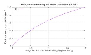
As long as the average hole size is a significant fraction of the average segment size, a substantial amount of memory will be wasted
