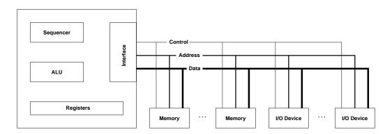
Today's common computer architecture uses busses to connect memory and I/O systems to the central processing unit (CPU)
