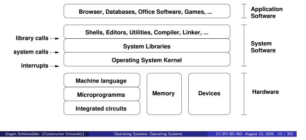
From the operating system perspective, the hardware is mainly characterized by the machine language (also called the instruction set) of the main processors, the memory system, and the I/O busses and interfaces to devices.
