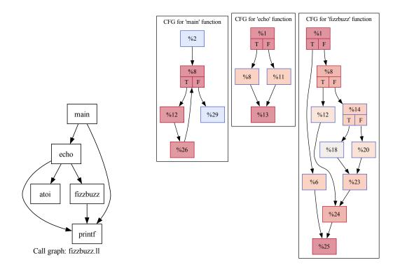
On the right, you see the control-flow graphs of the three functions. Nodes represent sequences of instructions and arrows possible jumps between these sequences of instructions.
